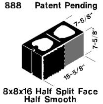
The 888 Half Split and Half Smooth block allows the mason to easily create a split face wall with an 8" smooth border around a truck dock door. By alternating 888's and 8" smooth halves he can create the vertical 8" smooth band needed for the dock seal. He then uses a standard smooth bond beam at the top to finish the 8" smooth band for the dock seal. This is the only block that allows for a normally bonded smooth band for a dock seal.
